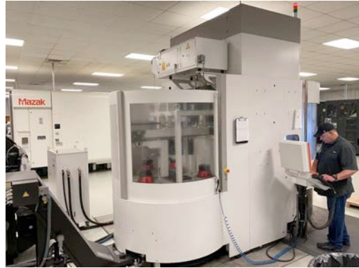
Jerry checking operation of Gray's DMG 5-axis machining center, with one of company's three Mazak 5-axis machining centers running unattended in background.
