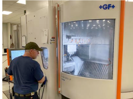
Mikron 5-axis machining center with seven pallets to support extensive unattended operation at Gray; company has four 5-axis Mikron machines; nearby sister division, Advanced Machining, has three more
