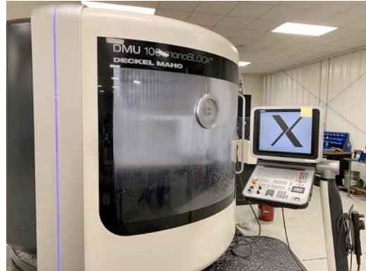
Gray's DMG 5-axis machining center in unattended operation manufacturing complicated titanium component for space customer
